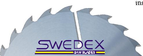
Wiper slot blades are Multi-rip blades. The wiper slots reduce the risk of getting stuck and also of the saw body becoming burnt. The guard tooth throws out loose cuttings and keeps the cutting groove clean. The blades can be used for sawing both green and dry wood.
