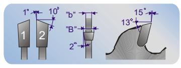
Universal saw blade, fine toothed with narrow cutting width. Suitable for ripping and cross-cutting of both hard and soft wood or thin board.
