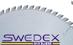
For Non-ferrous metals such as aluminum, copper and brass and also for plastics etc. Positive hook angle is used for automatic feed i.e. the material is gripped and negative used for manual feed.
