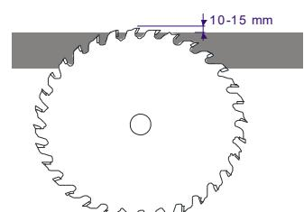
For thin, hard plastics we recommend alternately beveled teeth with chamfer (BAE).
