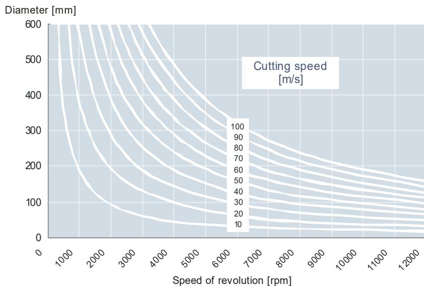
$$\text{Cutting speed} = \frac{\text{Diameter} * \text{RPM} * \pi}{60 * 1000}$$
