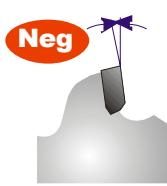
**Negative 2-5°** - cutting of metals with manual feed, plastics and laminates.
