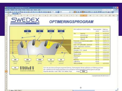
If the feed per tooth is very high the gullet volume needs to be calculated. A small gullet volume leads to an increased risk of cracks. We have developed a Microsoft Excel program for calculating the gullet volume along with other saw data. Contact Swedex technical sales people or one of Swedex resellers for assistance.
