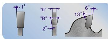
For panel sizing of laminated or non-laminated boards. Produced with long-life carbide tips. Left or right handed. Can also be manufactured with BA
