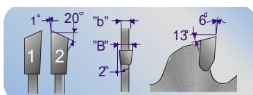
Close toothed saw blade for "Opti-cut" saws. Extra stable body. Differentiated tooth pitch together with copper rivets.
