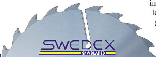
Wiper slot blades are Multi-rip blades. The wiper slots reduce the risk of getting stuck and also of the saw body becoming burnt. The guard tooth throws out loose cuttings and keeps the cutting groove clean. The blades can be used for sawing both green and dry wood
